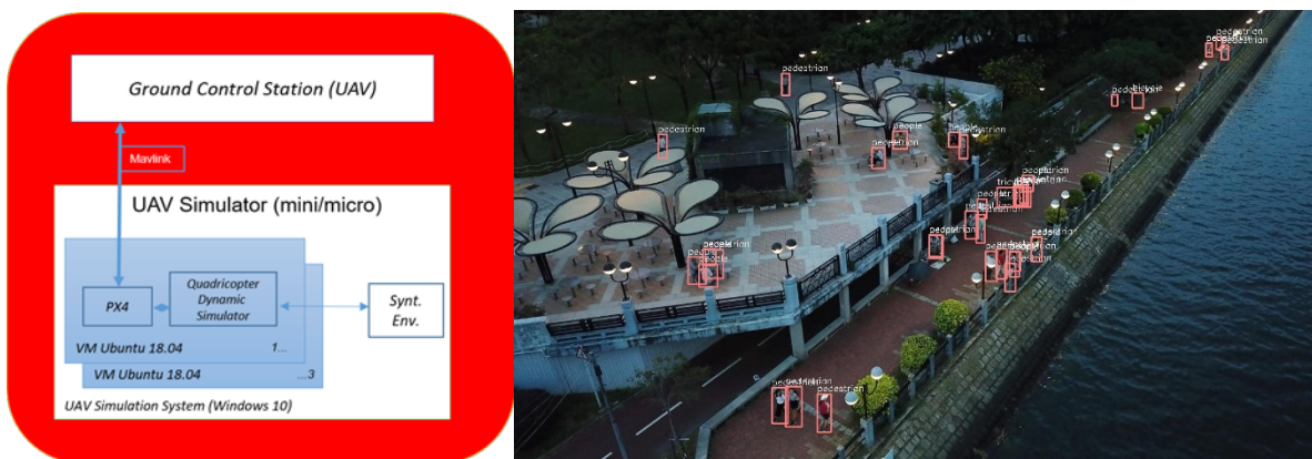
Figure 6: Left: Simulation System Architecture. Right: Example of annotations in visdrone dataset in a Multi-drone ISR Mission [14].
